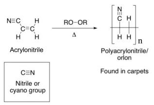
Polyacrylonitrile can form HCN if it is heated to decomposition.
