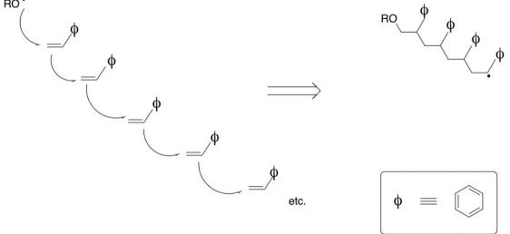
Divinyl benzene can be added as a cross-linker so chains link on both of its double bonds This make the copolymer more solid (as you encounter in many products) – typically about one part in 100 to one part in 6 of divinylbenzene may be added
