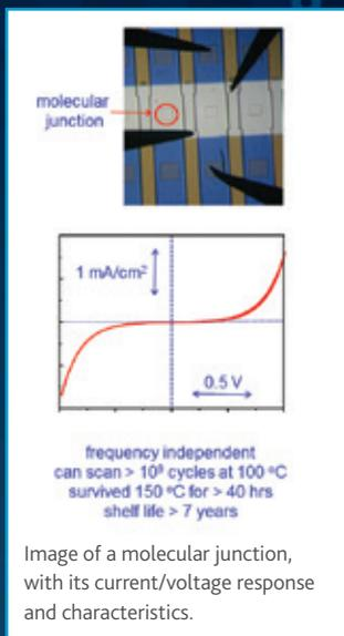
Image of a molecular junction, with its current/voltage response and characteristics.
