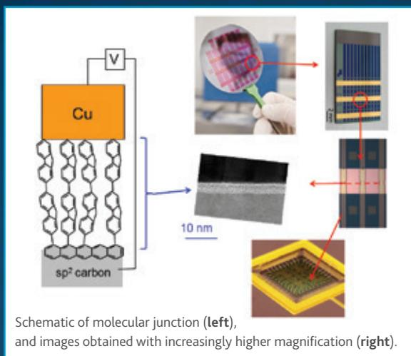
Schematic of molecular junction (left), and images obtained with increasingly higher magnification (right).
