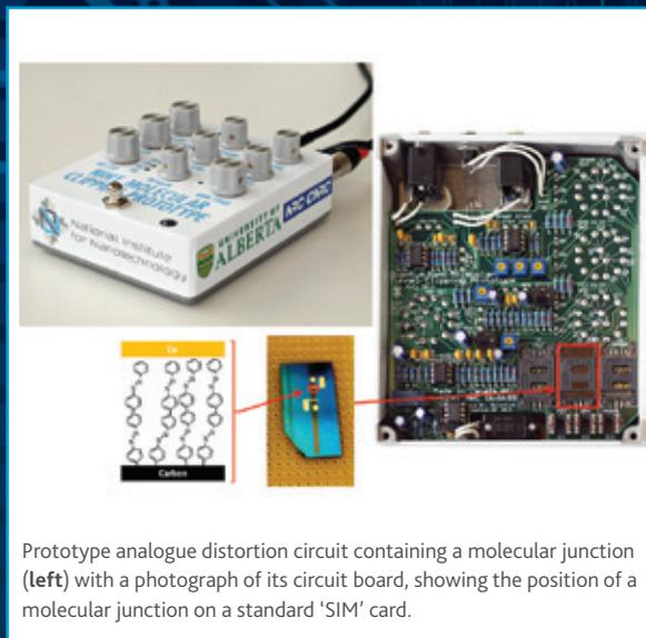
Prototype analogue distortion circuit containing a molecular junction (left) with a photograph of its circuit board, showing the position of a molecular junction on a standard 'SIM' card.
