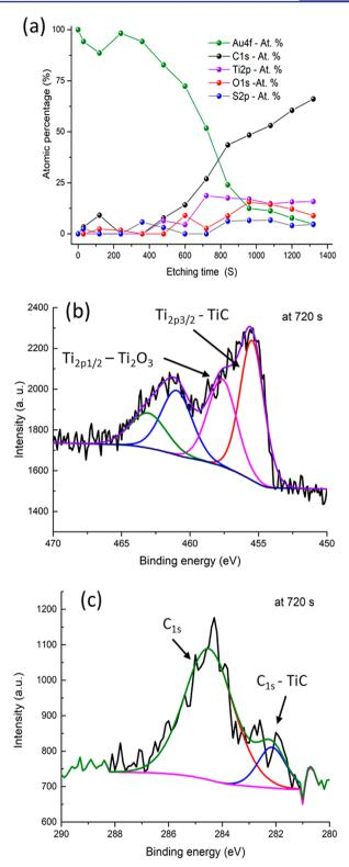
Figure 3. (a) Atomic percentages (%) vs etching time (s) for a Si/SiO<sub>2</sub>/PPF/BTB<sub>9</sub>/Ti<sub>2</sub>/Au<sub>20</sub> (b) titanium high resolution XPS signal, (c) carbon high resolution XPS signal.
