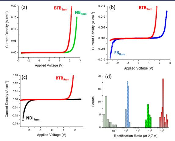
**Figure 4.** Current-density vs applied voltage (*JV*) curves for (a)  $Au/NB_8/Ti_2/Au$  (green curve) and  $Au/BTB_9/Ti_2/Au$  (red curve) MJ; (b) for  $Au/FB_8/Ti_2/Au$  (blue curve) and  $Au/BTB_9/Ti_2/Au$  (red curve); (c) for  $Au/NDI_7/Ti_2/Au$  (gray curve) and  $Au/BTB_9/Ti_2/Au$  (red curve) MJ. (d) Rectification ratio (*J*(+2.7 V)/*J*(-2.7 V) histograms for 63 BTB (red), 21 NB (green) and 42 FB (blue) devices and 26 NDI (gray) junctions.
