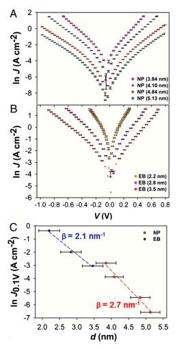
**Fig. 3.** Representative examples of J-V curves on a semilogarithmic scale for two molecules, NP (A) and EB (B). (C) Corresponding attenuation plots at 0.1 V [the length of the error bars in (C) are one standard deviation]. Junction area = 0.0013 cm<sup>2</sup>.
