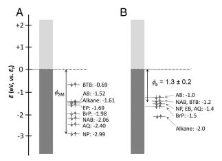
Fig. 6. (A) Energy levels before bonding the molecules to the carbon substrate where the hole transport barrier (defined as the negative of the given numbers) is defined by the Schottky-Mott rule ( $\phi_{SM}$ ), and spans a 2.3 eV range. (B)  $E_{\text{HOMO, onset}}$  energy measured using UPS for molecules bonded to PPF.
