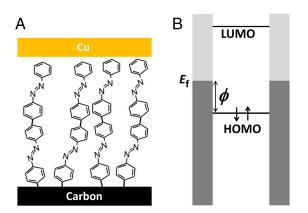
**Fig. 1.** (A) Schematic of a carbon/molecule/Cu junction with a multilayer of azobenzene. (B) Corresponding energy level diagram showing the Fermi level of the contacts offset from the molecular energy levels, where the closest occupied level (in this case the HOMO) represents a barrier for hole tunneling  $(\phi)$ . Filled orbitals in the contacts are indicated by shading.
