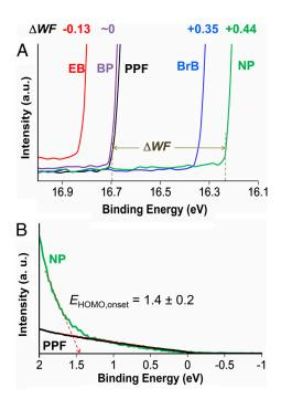
**Fig. 5.** (A) Close-up of the HBEC region for unmodified PPF and four samples modified with different molecular structures, showing that electron-withdrawing groups shift the WF positive, while a donating group shifts it negative. A detailed energy level diagram is given in *SI Appendix* (Section 4). (B) Example for determination of  $E_{\text{HOMO,onset}}$  using the method of Kim et al. (4). See *SI Appendix* (Section 3) for data for other molecules.
