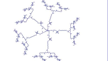
Bridged Pk dimer with an amine-terminated linker, activated as a squaric acid derivative, was linked to a five-fold scaffold made from a functionalized glucose molecule to give a pentameric presentation of trisaccharide dimers. Tetra- and tri-arm analogues based on glucose core were obtained by a similar sequence of transformations.
