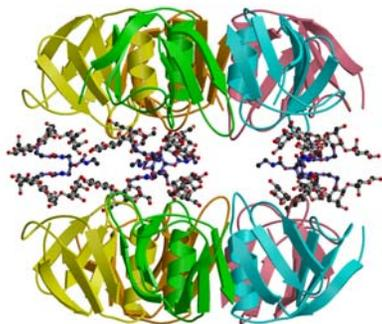
Figure 1. Crystal structure of 2:1 SLT-1/STARFISH adduct.
