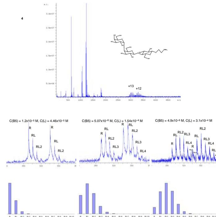
Figure 4. Different binding states of SLT-1B in complex with P<sup>k</sup>-trisaccharide. Actual spectra and 10 binding sites model ( $K_{D1} = 5 \times 10^{-4}$  M,  $K_{D2} = 5 \times 10^{-5}$  M).
