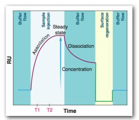
In principle, you could get a rough estimate of the  $K_d$  by plotting response (RU) as a function of sample concentration. However, this is not how it is typically done.
