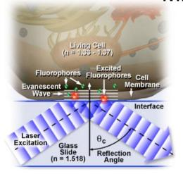
The energy of the evanescent wave is equal to the energy of that reflected light. Accordingly, the evanescent wave can be used to excite appropriate fluorophores to the excited state.
