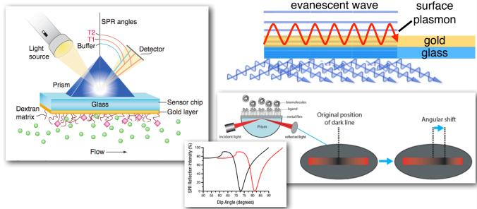
If the correct wavelength and angle is chosen, a resonant wave of excited electrons (plasmon resonance) is produced at the gold surface, decreasing the total intensity of the reflected wave. The angle of the SPR is sensitive to the layers attached to the gold. Binding and dissociation of ligand is sufficient to change the SPR angle.
