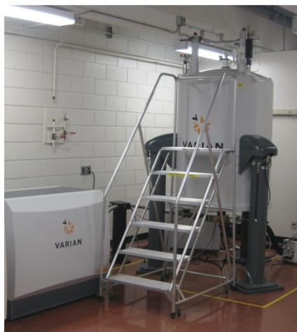
**The V700 NMR Machine Used for the Most Minute Samples**
