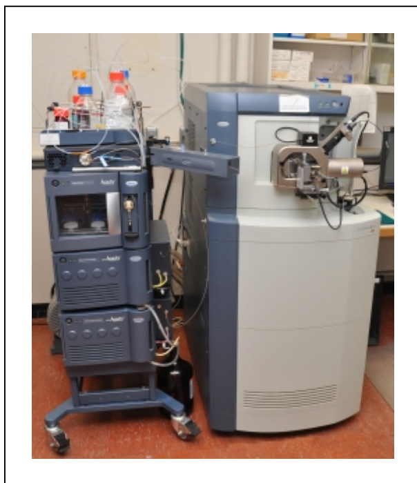
A Waters Q-TOF system with a nanoAcquity UPLC system and nano ESI ion source
